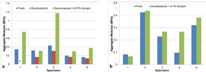
**Figure 1.** Effect of tissue processing on aggregate modulus of porcine articular cartilage. a - low genipin concentration; b - high genipin concentration. \*Data not available due to irregular stress relaxation profile.
