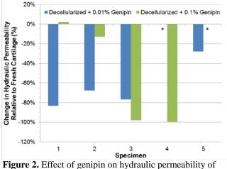
Figure 2. Effect of genipin on hydraulic permeability of porcine articular cartilage. \*Data not available due to irregular stress relaxation profile.
